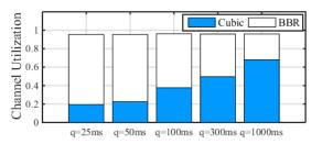
Fig. 1: Channel Utilization when one BBR flow shares the bottleneck with a Cubic flow.
