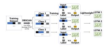
Figure 4: The process of training. All the training data go through clustering, then each cluster trains its own LSTM model.
