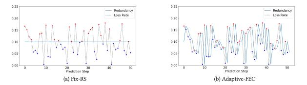
Figure 2: The packet loss rate predictions of the two traditional algorithms. The red dots means that the source packets cannot be completely recovered at that step, while the blue dots are the opposite.
