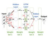
Figure 5: Compressing neural networks by weight pruning method. For each weight set, we sort the weights by their absolute values and remove them by masking to zero. The red lines represent the weights to be pruned.
