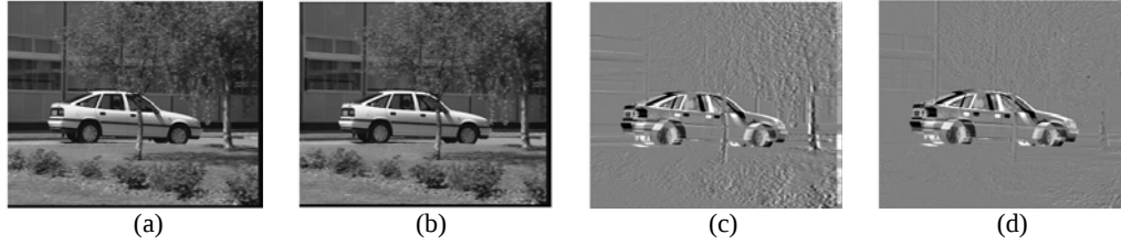
Fig. 4. VECTRA sequence. (a) Current frame (71 th frame). (b) Reference frame. (c) Difference image between (a) and compensated reference frame without selecting pixels. (d) Difference image between (a) and compensated reference frame with proposed algorithm.
