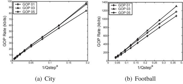
**Fig. 1.** The GOP rate characteristics with respect to the quantization step size of the key frame for test sequences: (a) City, QCIF ( $\alpha = 1.3$ ), (b) Football, CIF ( $\alpha = 0.8$ ).
