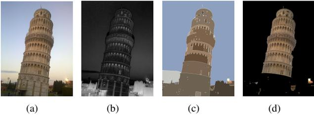
Fig. 2. An example of salient region segmentation. (a) Original image, (b) Saliency map, (c) Saliency segmentation, (d) Salient region.
