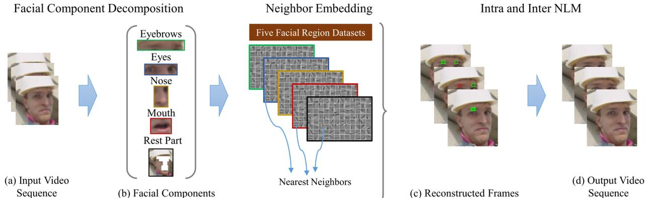
**Fig. 1.** An overview of the proposed method. (a) A LR input video sequence. (b) Facial components of each input frame are generated by facial component decomposition. (c) HR frames are reconstructed by neighbor embedding method with locality-constraint, then each frame is processed by Intra and Inter Nonlocal Means method. (The green blocks show the similar patches corresponding to the patch in the red block). (d) The output HR video sequence.
