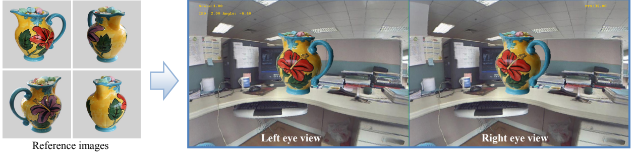
Figure 1: Stereo visual hull rendering result using our improved pipeline. With 47 input reference images, a rendering speed of about 30 fps can be achieved on a double-GPU personal computer.
