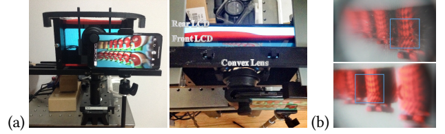
Figure 5: (a) The setup of our hardware prototype. (b) The light field display results captured by a camera (top: front focus; bottom: rear focus).
