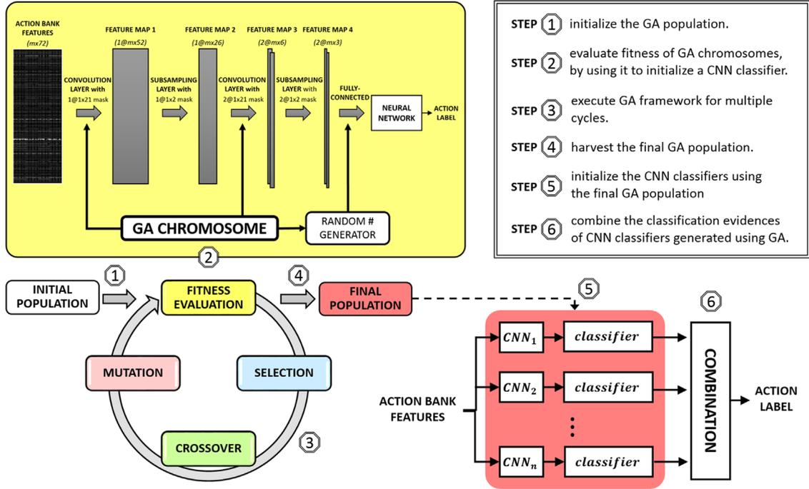
**Fig. 1.** Overview of the proposed classification system. The various steps involved in the proposed approach are numbered and a short description of each step is given on the top right corner. Best viewed in color.
