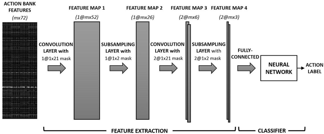
Fig. 4. Architecture CNN classifier for human action recognition.
